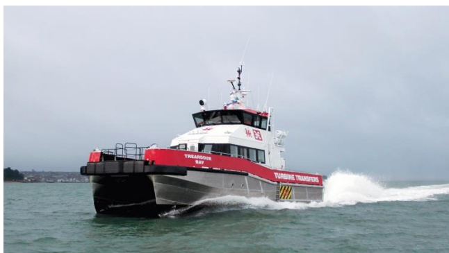
Crew Transport Vessel equipped with two Voith Linear Jets (VLJ)
