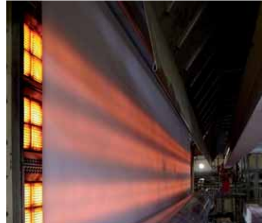
Perfect drying capacity due to contactless infrared drying.
