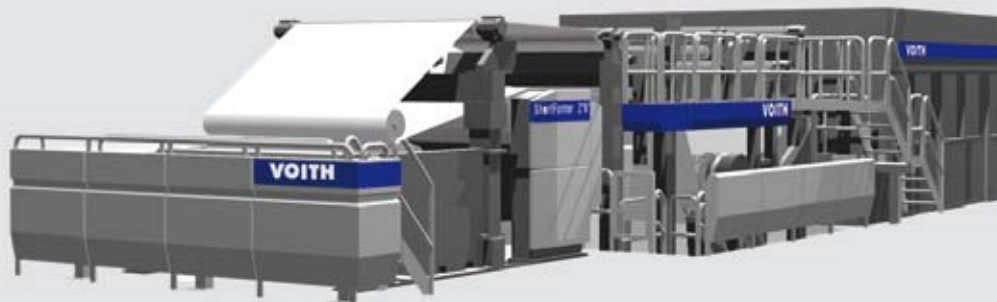
In a special Voith Paper machine for banknote paper, the MasterVat and ShortFormer B are used for the double-ply sheet forming.
