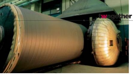
Fig. 3: Forming roll covered with Diamantite put into the curing chamber for Andritz AG, size of the roll: 1500 x 1512 x 3300 mm.
