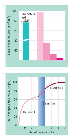
most effective modules, i.e. with flotation and dispersion, is required. With a residual load of 200 ppm and a cleanness target of 10 ppm, the efficiency must be increased by an additional 95%. This corresponds to three additional modules with an individual efficiency of 65% each.
