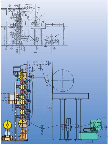
*Fig. 6* shows the original situation and *Fig. 7* the final condition of the calenders.
