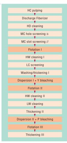
The initial dirt load in *Fig. 9* was 1400 ppm. The first significant increase in cleanness is obtained with Flotation I, whilst the second increase is with Dispersion I including reductive bleaching. Then follow noticeable reductions after Flotation II and Dispersion II.
