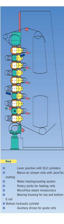
Fig. 1: Different Janus calender lay-outs, 1 x 6 rolls, 2 x 5 rolls, 2 x 7 rolls, 1 x 11 rolls.
