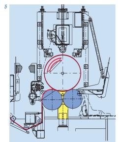
a single drum winder had to be used. The reason for this were the nip forces resulting from the great roll weights which, with the two drum winder, could lead to winding faults, such as crepe wrinkles, breakages, excessive stretch etc. *Fig. 3* shows an example of 2 types of paper on this subject.
