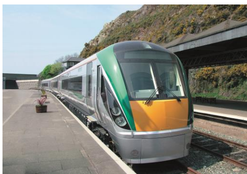
Irish Rail 22000 class diesel railcars, equipped with turbo transmission, cooling system and Scharfenberg coupler.
